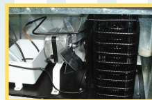
Condenser that is less prone to blocking with dust
